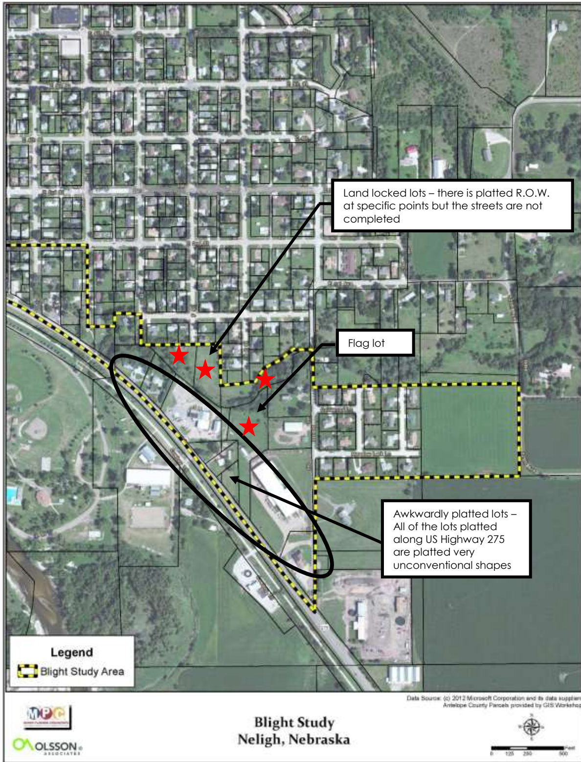
Figure 8B Faulty Lot Layout Conditions
